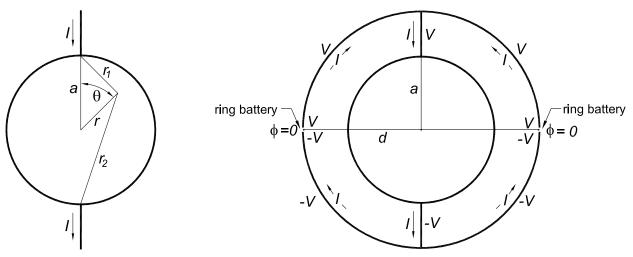
Suppose the wires have radius  $b \ll a$ , and their surfaces of contact with the bead are equipotentials, to show that the resistance of the bead is that of a piece of wire roughly b long, if that wire also had conductivity  $\sigma$
