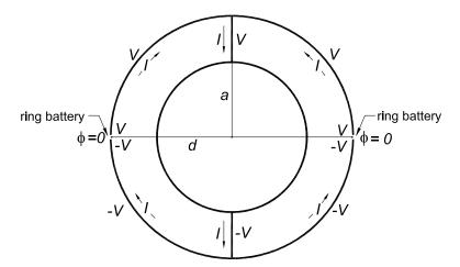
In the region a < r < d and outside the wires at  $\theta = 0$  and  $\pi$ , the potential obeys  $\nabla^2 \phi = 0$ , is azimuthally symmetric, and symmetric about the plane  $\theta = \pi/2$ , so it can be expanded as,
