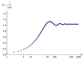
The numerical evaluation converges to  $\approx 1.05 I/\pi\sigma b$  after roughly N = 2a/b = 67 terms, while sec. 2.2 indicates that the value should be  $I/2\pi\sigma b$ . In my view, while the numerical
