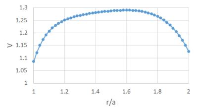
The potential outside the perfectly conducting hemispheres, which are held at potentials  $\pm V$ , is given in eq. (3.36) of [2]. In our notation,
