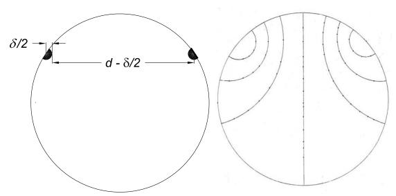
We note that the current and the electric field must be tangential to the edge of the disk. We recall that the equipotentials of eq. (4) are circles, as shown in the figure on the right above (from Kirchhoff), and that the corresponding electric field lines are also circles which,
