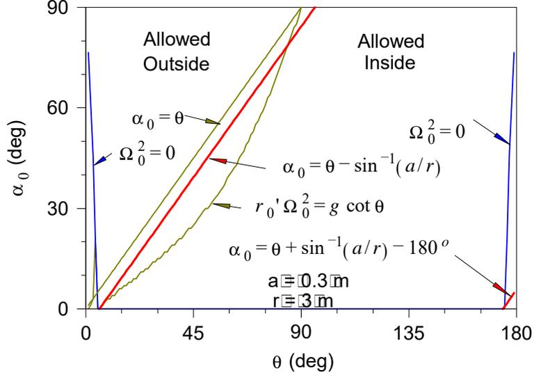
Figure 6: The allowed values of the tilt angle  $\alpha_0$  as a function of the angle  $\theta$  of horizontal orbits for the conditions of Table 1. The allowed region is bounded by four curves, derived from expressions (2), (50) and (56).
