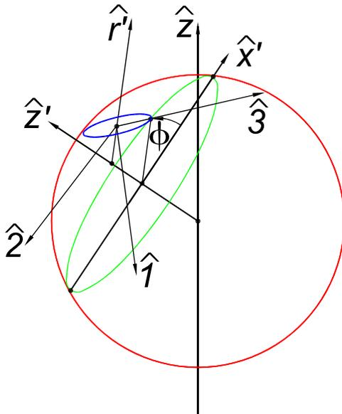
Figure 2: The azimuth of the point of contact of the disk with the sphere to the  $x'$ -axis is  $\phi$ . The unit vector  $\hat{\mathbf{r}}'$  is orthogonal to the  $z'$ -axis and points towards the center of the disk (or equivalently, towards the point of contact). Unit vector  $\hat{\mathbf{2}} = \hat{\mathbf{3}} \times \hat{\mathbf{1}} = \hat{\mathbf{z}}' \times \hat{\mathbf{r}}'$ .
