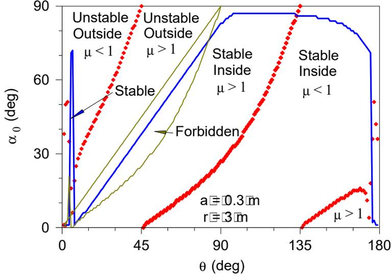
Figure 7: The regions of stability in the  $\alpha_0$ - $\theta$  plane of small oscillations of a hoop of radius  $a = 0.3$  m inside or outside a sphere of radius  $r = 3$  m, according to eq. (80). Orbits are forbidden inside the crescentlike region near  $\alpha_0 = \theta$ , according to eqs. (60) and (82). The regions where a coefficient of friction  $\mu$  greater or less than unity according to eq. (60) are also shown.
