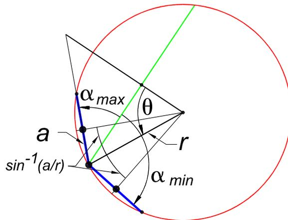
Figure 3: Geometry illustrating the extremes of angle  $\alpha$ .
