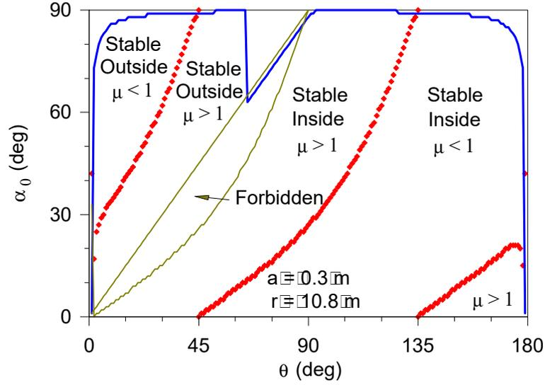
Figure 8: The regions of the  $\alpha_0$ - $\theta$  plane for which horizontal orbits are stable, and for which the required coefficient of friction is greater or less than 1, for a hoop of radius 0.3 m either inside or outside a sphere of radius 10.8 m.
