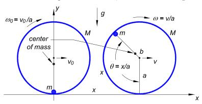
Taking the origin of an x-y coordinate system to be at a point of contact of the tire with the road when mass m is at its lowest position, when the point of contact is at x the geometric center of the tire has horizontal velocity v and the center of mass of the unbalanced tire has rotated through angle  $\theta = x/a$ . The angular velocity  $\omega$  of the tire is,
