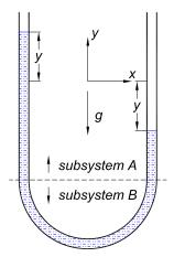
Designate the water in the vertical arms of the U-tube as subsystem A, and the water in the half-circle arc of the tube as subsystem B. Discuss the horizontal components of the velocities of the center of masses, and of the momentum, of the two subsystems (whose masses are equal). Do the subsystems contain hidden momentum,  $P_{\text{hidden}}$ , defined by,
